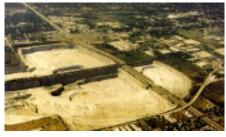
Thornton Composite Reservoir Final Prep RME provided Structural Engineering services for almost all the structural components of the project, including approach slab, drop shaft, portal, tunnels, plunge & deaeration structure tunnel plugs. This Reservoir is part of the MWRDGC's Tunnel and Reservoir Plan (TARP).
